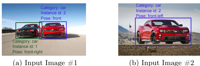
Fig. 1. Object co-detection for two images. The goal is to i) detect objects; ii) identify which objects correspond to the same object instance (e.g. the red Camaro); we call these instances matching objects ; iii) estimate the viewpoint transformation between matching objects.
