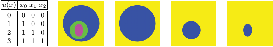
Fig. 3. Label Representation: Labels between 0 and k (here: k = 3 ) can be represented by k binary variables [15]. All these binary variables fulfill the logical conditions x_\ell \Rightarrow x_{\ell-1} (left table). This relationship is illustrated in the four images for u(x) (left image) and x_0, x_1 and x_2 (from middle to right).
