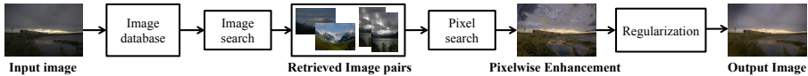
Fig. 2. Overview of the proposed coarse-to-fine local enhancement method. Enhancement maps are contrast enhanced for better visibility.
