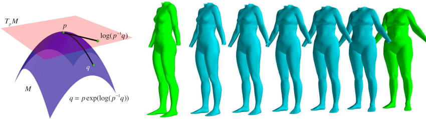
Fig. 3. Smooth Manifold. (left) T_pM is a tangent space to M at p . T_pM and M are connected via \exp and \log . (right) Interpolation (light blue) along a geodesic path between two human shapes p and q (green)
