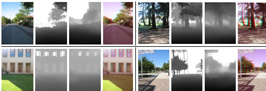
Fig. 8. Single image results obtained on test images from the Make3D dataset. Each result contains the following four images (from left to right): original photograph, ground truth depth from the dataset, our inferred depth, and our synthesized anaglyph - image. The depth images are shown in log scale. Darker pixels indicate nearby objects (black is roughly 1m away) and lighter pixels indicate objects farther away (white is roughly 80m away). Each pair of ground truth and inferred depths are displayed at the same scale.
