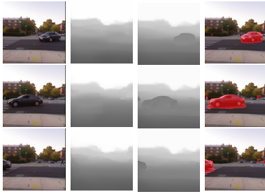
Fig. 4. Importance of temporal information. Left: input frames. Mid-left: predicted depth without temporal information. Note that the car is practically ignored here. Mid-right: predicted depth with temporal information, with the depth of the moving car recovered. Right: detected moving object.
