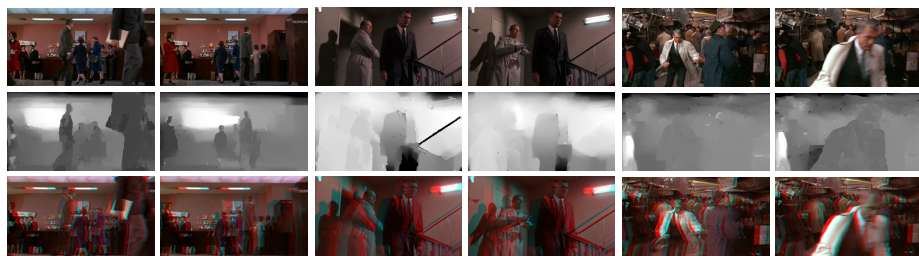
Fig. 11. Several clips from the feature film Charade . Each result contains (from top to bottom): the original frames, estimated depth, and estimated anaglyph - automatically generated by our algorithm. Some imperfections in depth are conveniently masked in the 3D image due to textureless or less salient regions.
