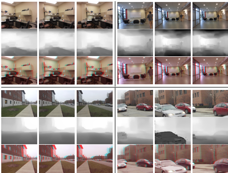
Fig. 7. Results obtained on four different sequences captured with a rotating camera and/or variable focal length. In each 3 \times 3 block of images, we show the input frames ( top ), inferred depth ( middle ) and inferred 3D anaglyph ( bottom ). Notice that the sequences are time-coherent and that moving objects are not ignored.
