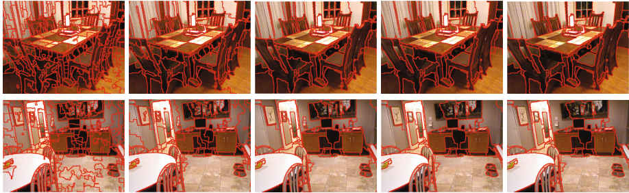
Fig. 4. Segmentation Examples. We show two examples of hierarchical segmentation. Starting with roughly 1500 superpixels (not shown), our algorithm iteratively merges regions based on the likelihood of two regions belonging to the same object instance. For the final segmentation, no two regions have greater than 50% chance of being part of the same object.
