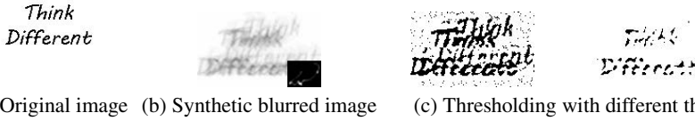
Fig. 2. Difficulty of applying the segmentation (text binarization with thresholding) technique to a blurred text image.
