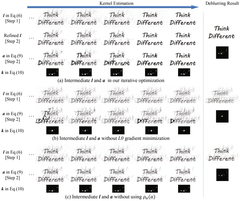
Fig. 6. Effects of L_0 gradient minimization and \rho_a(a) . (a) intermediate l and a in our algorithm at a coarse level; (b) intermediate l and a at the same level without L_0 gradient minimization; (c) intermediate l and a at the same level without using \rho_a(a) in Eq. (7)
