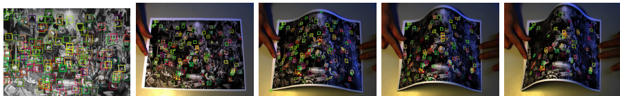
Fig. 7. Keypoints recognition and pose estimation on the video with severe bending deformations. The first image is the model image and the rest are example frames.
