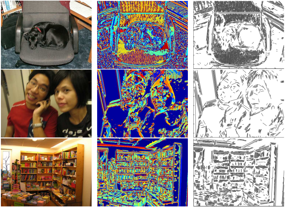
Fig. 1. Self-similar sketches. The figure shows a few example images, the quantised local descriptors, and the fitted line segments constituting the sketch. The calculation is straightforward and relatively efficient.
