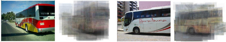
Fig. 4. Visualizing images (left) in terms of their most discriminative patches (right). The patch detectors were fired on a novel image and the high-scoring patch detections were averaged together, weighted by their scores.
