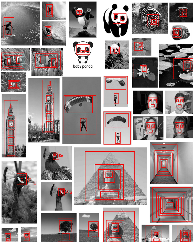
Fig. 6. Example matching of nested pictorial structures. We select 12 categories of images from Caltech256, see [26]. Each category is divided into separate sets for training and testing. In the training step, we ask a user to mark a number of nested rectangular windows on each training image, and a linear SVM classifier is trained for each category from both positive and negative samples using nested feature descriptors. The feature descriptor of each part is a concatenation of histogram of gradients and colors in that part, excluding histograms associated to any child parts. In the matching step, the normal vector derived from the trained linear SVM classifier is used to obtain the per-pixel cost of Equation (9). The matching is performed on images from the test set for each category. Similar to the recognition framework of Felzenszwalb et al. [13], we build an image pyramid of 10 levels ranging from twice the size of the original image to half of the original image size. Matching a nested pictorial structure is then performed on each derived image and the one that receives the minimal cost is selected and reshaped back. In some images the rectangles are attached to a single object. In others the rectangles include multiple objects and their surrounding context (e.g. clown fish and anemone, the Sphinx and pyramid, etc).
