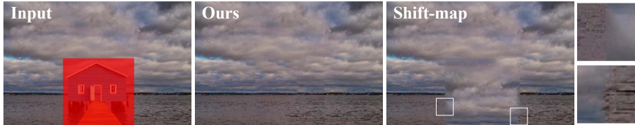
Fig. 17. Comparison with Shift-map [15]. In the zoom-in we show how Shift-map behaves near inconsistent seams. This result is obtained from the authors’ demo [21]. We have tried various parameter settings but observed similar artifacts.
