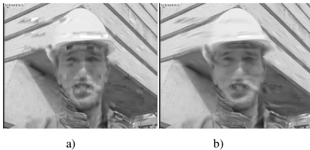
Fig. 5. Error distribution: bursty. Concealed image Intra of “Foreman” with the: a) FSE weighted 0.1, Y-PSNR=26.84dB; b) Our method, Y-PSNR=27.25dB.
