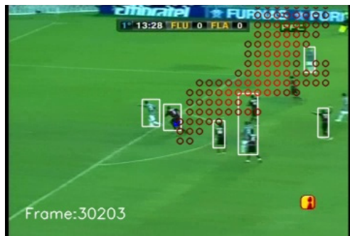
Fig. 4. Frame identified as a highlight. The higher the value of the convergence, the redder is the circle. This image also contains the players boxes and the blue arrow at the center representing the camera velocity. This frame is within the sequence shown in Fig.3.
