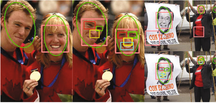
Fig. 2. Face detection examples based on \mathbf{F} (left) and \mathbf{FC2FFs} (right). They illustrate the benefits of the integration of facial features detectors, serving to remove false detections (upper row) and undetected faces located by its facial features (bottom row).
