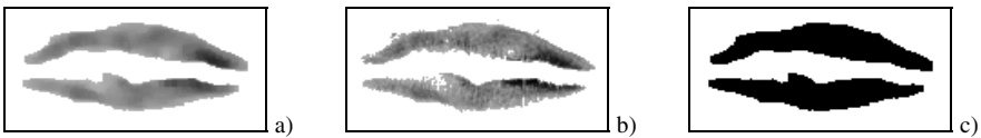
Fig. 1. Steps of lip area detection: a) the image after evaluating pixels against a threshold, b) after blurring, c) the detected lip area
