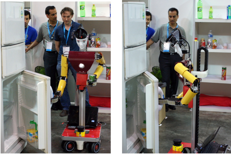
Fig. 1. Our domestic service robot Dynamaid opens and closes the fridge at RoboCup 2010 in Singapore
