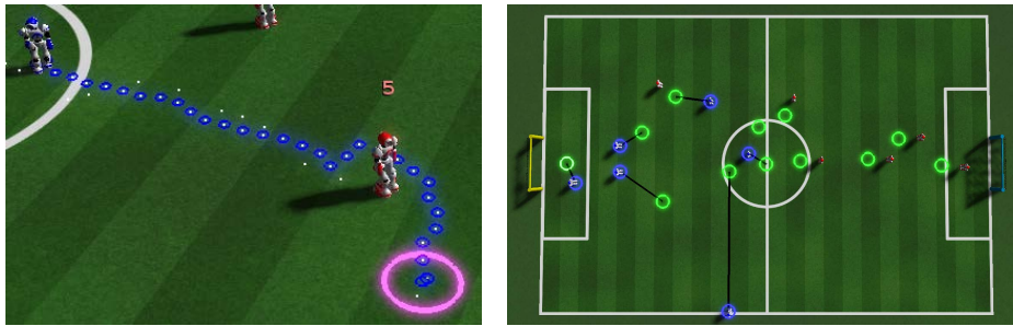
(a) Path planning: A single agent's path plan is laid out as a series of blue circles; the white points indicate other considered routes. In this example, the agent anticipates a collision with an opponent player and schedules the path accordingly.
