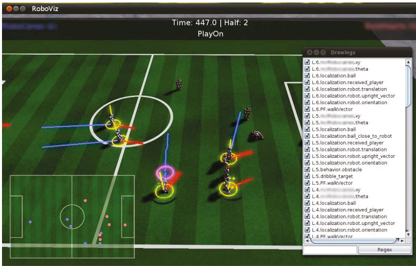
Fig. 2. The current user interface includes the same game state information as the 3D monitor; however, it also has an optional 2D aerial view, a panel for filtering drawings, an agent-perspective camera
