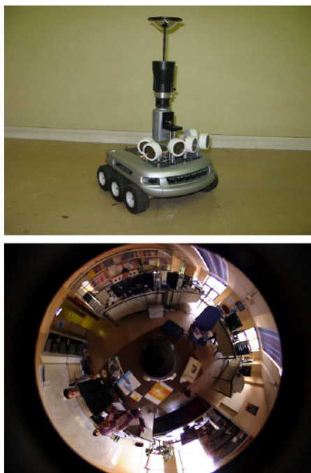
Fig. 2. Top: omnidirectional sensor embedded on a mobile robot. Bottom: omnidirectional image.
