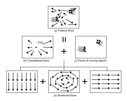
**Fig. 3.** Components of feature flows. Intersection point of translational flow (b) corresponds to Focus of Expansion (FOE) and it indicates direction of camera movement. However, feature flows computed from egocentric video (a) include flows caused by independently moving objects (c) and rotational movements (d). Components corresponding to (c) and (d) must first be separated from computed flow (a) to estimate FOE of input frame.
