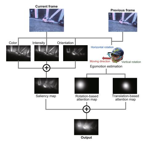
**Fig. 1.** Flow for our proposed framework. While bottom-up visual saliency maps are computed from input egocentric video, motion maps are computed using person's egomotion. These additional motion maps are integrated into visual saliency maps, and resulting map achieves higher accuracy in predicting human attention.
