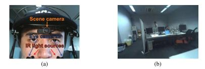
**Fig. 6.** (a) Mobile gaze tracker employed in experiments. Scene camera is installed and it captures egocentric video of subject at 30 [Hz]. Two eye-cameras and two infrared light sources can record ground-truth gaze points on egocentric video at 240 [Hz]. (b) Example frame of egocentric video. Horizontal field of view of scene camera was  $121^{\circ}$ , and resolution of egocentric video was  $640 \times 480$  [pixels].
