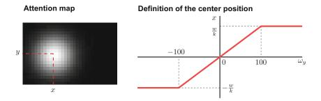
**Fig. 2.** Rotation-based attention map. 2-D Gaussian circle is drawn with fixed variance to generate rotation-based attention maps based on angular velocities. According to report by Hillair et al. [10], center of Gaussian is defined so that it is proportional to angular velocity within the range of 100[deg /s].
