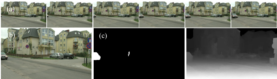
Fig. 9. The 77 th frame in the data set “Poznań”. (a) The reference frames. (b) The current frame. (c) The white region is the detected moving object. (d) Final depth map.
