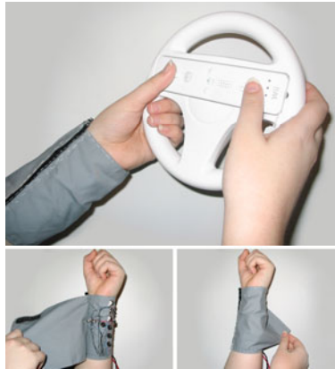
Fig. 1. The Gauntlet Guide coupled with the Wii Wheel. The bottom two photos show how the actuators are covered.
