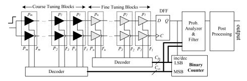
Fig. 8. The complete TRNG system
