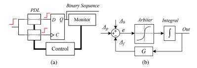
Fig. 5. The TRNG system model
