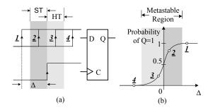
Fig. 4. (a) Flip-flop operation under four sampling scenarios, (b) probability of output being equal to '1' as a function of the input signals delay difference ( $\Delta$ ). The numbers on the probability plot correspond to each signal arrival scenario.
