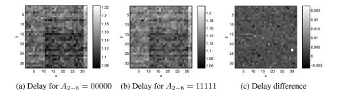
**Fig. 10.** The measured delay of  $32 \times 32$  circuit under tests containing a PDL with PDL control inputs being set to (a)  $A_{2-6} = 00000$  and (b)  $A_{2-6} = 11111$  respectively. The difference between the delays in these two cases is shown in (c).
