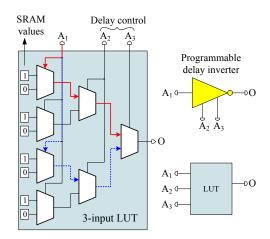
Fig. 3. Precision PDL using a single LUT
