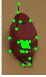
Fig. 3. Features are not uniformly distributed over the object and the center of gravity of the key points does not coincide with the center of gravity of the object. The small dots represent the features and the big dot represents their barycenter. The figure is better visualized in color.
