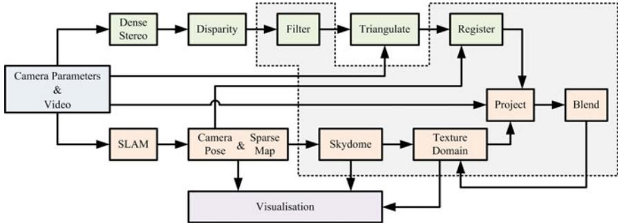
**Fig. 1.** Processing pipeline of the proposed method. Video images are processed independently by SLAM and dense-disparity until they are registered to each other. Projection blends surface detail and video colour into texture maps used for visualisation. This paper addresses mainly components enclosed in the dashed box.
