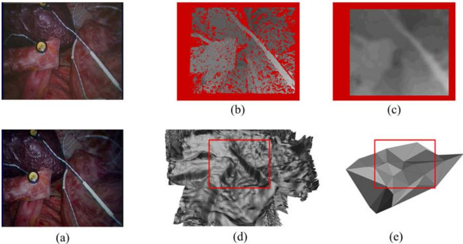
**Fig. 3.** Stereo disparity and estimated dense surface. a) shows left and right video frame of the phantom sequence; b) shows raw stereo disparity; c) filtered and smoothed disparity; d) shows the flat-shaded highly tessellated  $Y'$  with the red rectangle marking the part that would be covered by the video frame. For comparison, the sparse SLAM map surface  $Y$  is shown in e).
