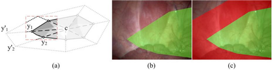
**Fig. 2.** Padding the SLAM-map with additional triangles. b) and c) illustrate the effect in the video image with green being the original sparse SLAM-map and red the additional area covered by the skydome.
