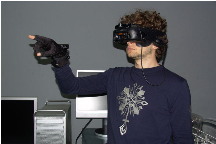
Fig. 4. See-Through HMD, datagloves and head/wrists wireless trackers worn during testing
