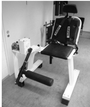
Fig. 1. Adjustable knee joint torque measuring device
