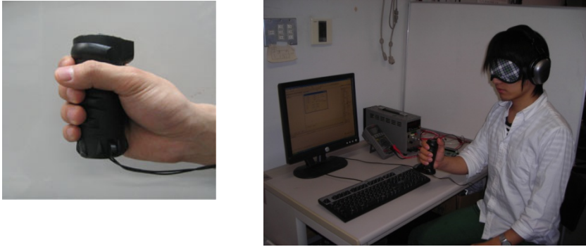
Fig. 1. Experimental setup and environment. (a) The VAI used in the experiment. (b) Experimental environment A vibration motor is mounted inside the vibration device.
