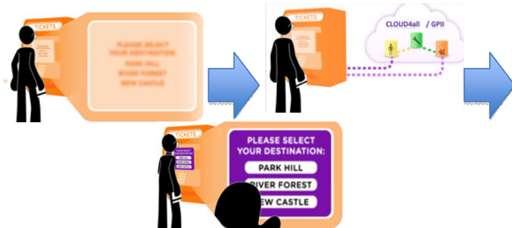
Fig. 2. With GPII the interface will adapt to the user automatically based on the user needs profile on a card or in the cloud, in this case providing a larger, higher contrast display.
