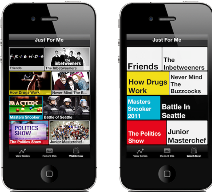
Fig. 5. Screen shot of TV guide prototype showing shortlisted content based on shared user model (left), low vision optimised version of the interface (right)
