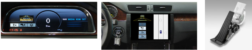
Fig. 7. HAVEit Display in the instrument cluster (left) and on an additional touch screen (middle) and accelerator pedal for haptic feedback in the HAVEit ARC demonstrator
