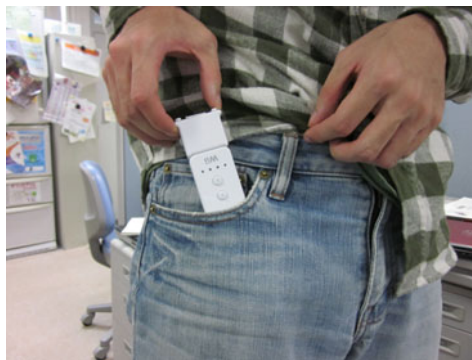
Fig. 1. Appearance of sensor position. We plan to activate incident detection application only when mobile phone is in bottom of user's pocket. Bottom of user's pocket can be expected not to have considerable individual difference in shape.
