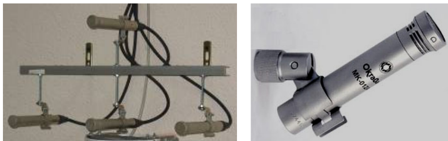
Fig. 2. Model of microphone array (left); one microphone of the array (right)
