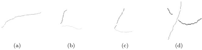
Fig. 6. Closer examination of segment joining results: (a) Segments recognized as a straight fiber; (b) Segments recognized as separate fibers; (c) Segments recognized as two separate straight fibers; (d) Segments from overlapping fibers recognized as a straight and a curved fiber
