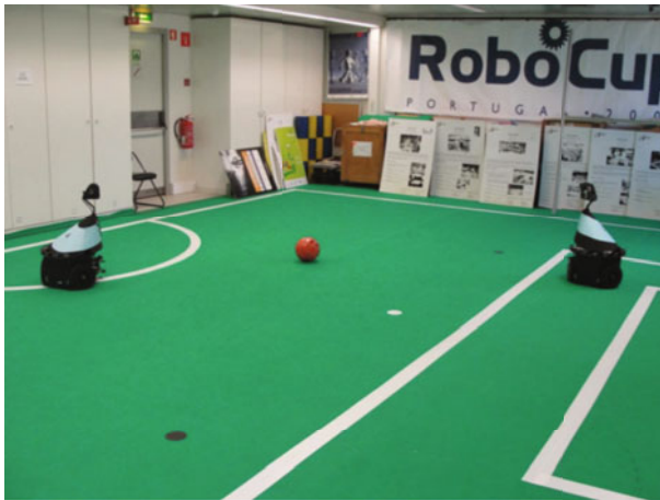
Fig. 5. Real robot example for one of the layout locations: the robot on the left is the robot that informs about the ball position, while the robot on the right is the kidnapped robot, in location 4
