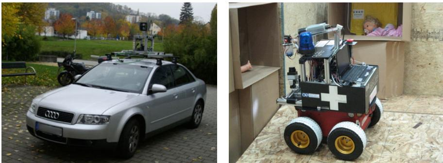
(a) Velodyne HDL-64E mounted on a (human driven) street car. (b) 3D LRF mounted on our autonomous rescue robot Robbie.
