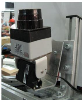
(a) Laser scanner mounted on two servo motors.
