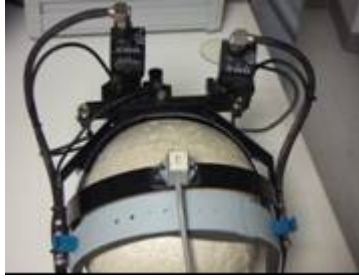
Fig. 5. Magnetic sensor attached to the ASL eye tracker's helmet
