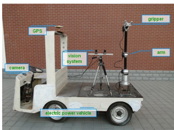
Fig. 1. Components of the robot
