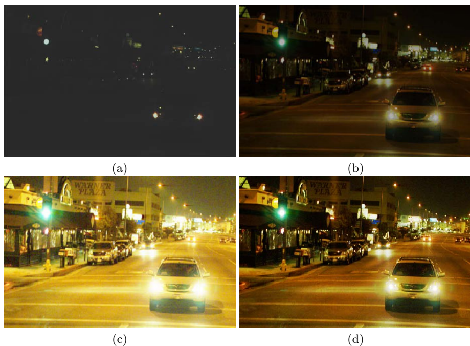
Fig. 4. (a) the original image before Gamma correction, (b) after Gamma correction, (c) Gamma correction followed by histogram equalization, and (d) joint Gamma correction and contrast-tone optimization by the proposed method
