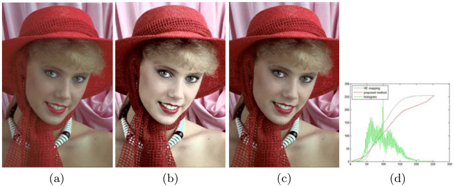
Fig. 3. (a) the original, (b) the output of histogram equalization, (c) the output of the proposed method, and (d) the transfer functions and the original histogram
