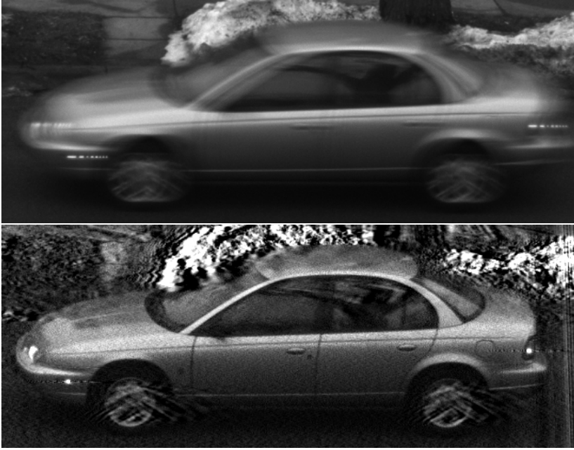
Fig. 6. (Top) Flutter shutter image captured of a car driving down a residential street, with 43 pixels of blur. (Bottom) Reconstructed image, in which details on the car are preserved; note that the static background has artifacts from the deconvolution. In this case, the street's speed limit serves as a strong prior on object velocity, obviating the need for explicit pre-capture velocity estimation. Exposure time is 20ms with velocity of 1.1 pixel per ms; shutter sequence is 1001001001100110001000111100011111111, with t_{chop} = 1ms .
