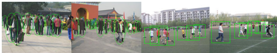
Fig. 1. Some combined results of Structural Filter approach to detect occluded pedestrian and articulated human
