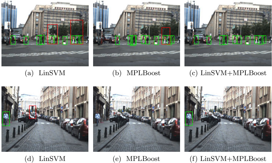
Fig. 2. MPLBoost and SVMs perform well but tend to have different false positives (a,b,d,e – red boxes correspond to false positives). By combining both classifiers the false positive rate can be reduced (c,f).
