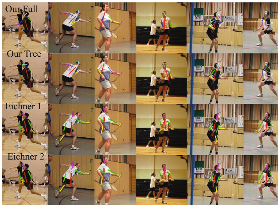
Fig. 3. Examples of stick-figure, upper body parses of figures in our dataset produced by the full model trained on our dataset top row, our tree model top-center and the code of Eichner et al. bottom center (trained on buffy_2to6) and bottom (trained on buffy_3&4 and pascal), all applied to our dataset. Red: upper body; Green: head; Blue-Purple: left upper/lower arm; Green-Yellow: right upper-lower arm. Note doubled arms produced by the tree model and a tendency for Eichner et al. to produce hanging arms, most likely a result of the strong geometric prior in their training datasets.
