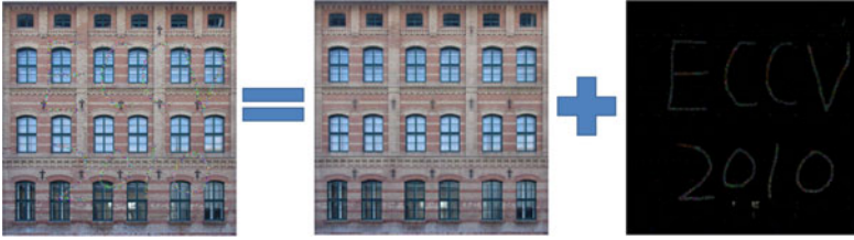
Fig. 1. Result of our method on a color facade (left). The method automatically seek a low dimensional representation (middle) and separate the sparse irregular patterns (right). Better viewed in color and zoom in for details.
