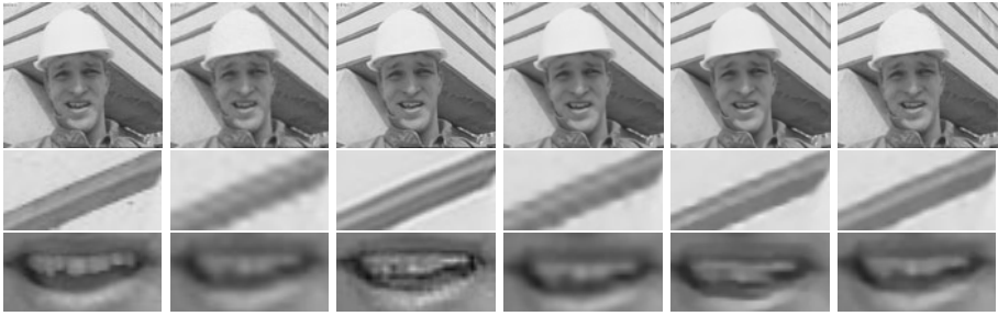
Fig. 6. Video super-resolution for Foreman sequence (frame 8, zoom factor 3, PSNR and SSIM in brackets). Left to right: Ground-truth, BI(30.1758, 0.8739), GNL-Means(33.2233, 0.9041), BM3D(33.45, NA), 3D-KR(33.30, NA), NL-KR( 33.7589 , 0.9137 ). GNL-Means performs well at regular-structured area but generates severe block artifacts where few similar patches can be found; BM3D suffers from jagged effects at edges; 3D-KR can not preserve the straight structure well due to the non-robustness of its spatial-temporal kernel and can generate ghost image ; our method preserves both the larger structure and fine details well and is free of these artifacts.
