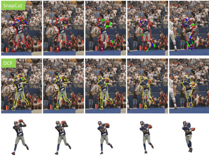
Fig. 7. The football sequence, from left to right: frames 2, 5, 10, 13, 20. Frame 1 is pre-segmented. First row: segmentation ( red curves ) and user scribbles ( blue as foreground and green as background ) by the SnapCut system. Second row: segmentation ( yellow curves ) and user scribbles by our system. Third row: new composites on white.
