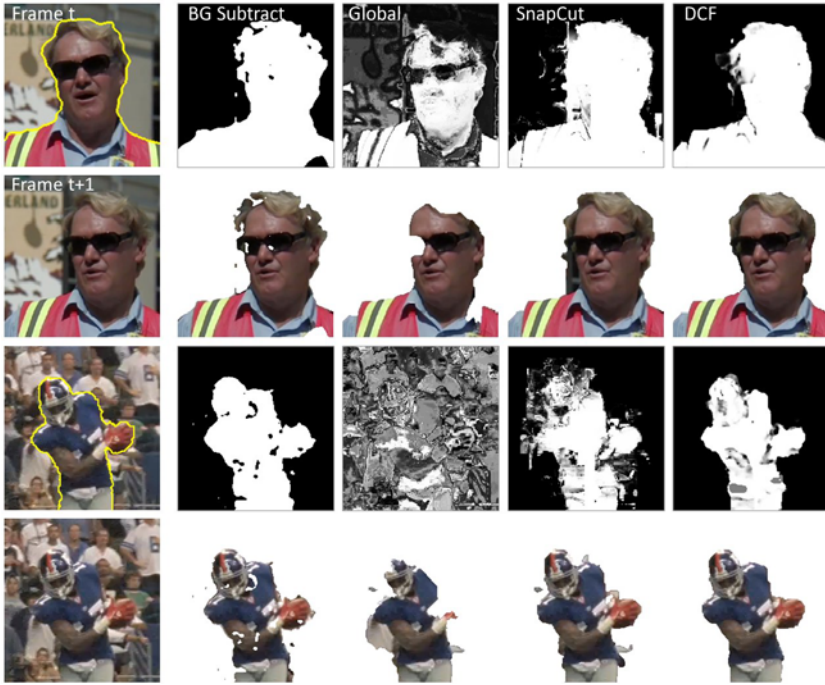
Fig. 6. Comparing color probability maps and segmentation results generated by simple background subtraction, the global GMM color model, the local color model from [7], and the proposed DCF on two examples. The gray scale images are the color probabilities generated by each method followed by their corresponding segmentation results. (For better visualization, images are cropped from original videos. See figures 3 and 7 for the full frames.)
