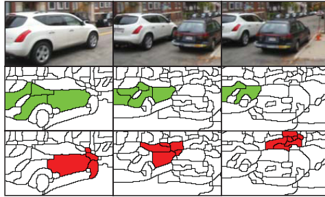
Fig. 3. Two hypotheses that are incompatible. The hypotheses (shown in green and red) overlap on the first two frames. The segmentation of the sequence should ensure their exclusive selection. MHVS ranks hypotheses photometrically and penalizes the non-consistent selection of the most coherent ones over time.
