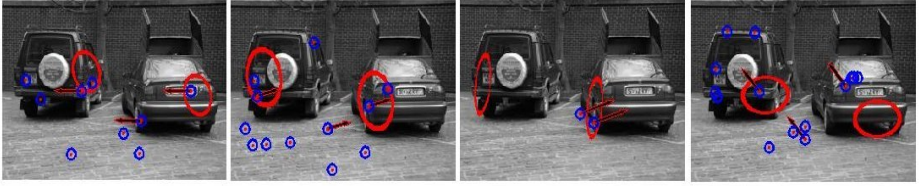
Fig. 2. Each image shows a Part R_j^k (Red Ellipse) with the set of candidate locations x_j^k . Locations with high belief are those who vote and are drawn with an arrow pointing to the object center. The beliefs generated by the graphical model form a strong constraint on the voting pattern of Part candidates so that only those locations who have global shape support end up voting. The images contain multiple instances thus the belief pattern of P(x_j^k) is multi-modal. Candidate locations from both object instances end up voting.
