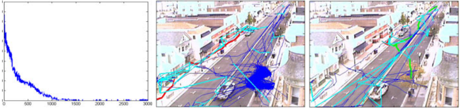
Fig. 6. (a) Boosting algorithm decreases linkage classification errors as increasing number of weak classifiers are learned. The x-axis shows the progress of boosting learning as the number of weak classifiers, and y-axis shows classification error. Detected links overlaid (in cyan) on sequences of (b) a postman and (c) a delivery truck.
