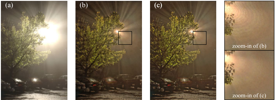
Fig. 5. Quantization artifacts of O(N) time bilateral filter. (a) Input HDR image (32bit float, displayed by linear scaling). (b) Compressed image using the O(N) bilateral filter in [15] (64 bins). (c) Compressed image using the guided filter. This figure is best viewed in the electronic version of this paper.
